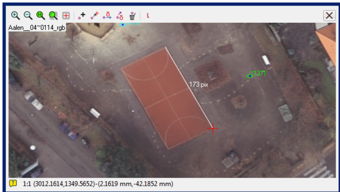
Fig. 88. Distance measuring in the “Points measurement” module
