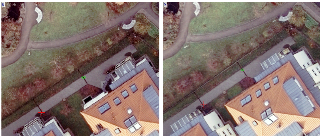
Fig. 144. The left image shows triplet point, located in the center of triple overlap area, the right one – triplet point from the right image
