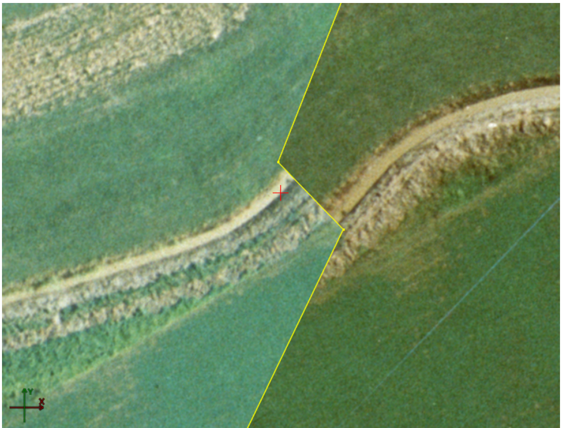
Fig. 77. The elements of an extended object (road) are poorly aligned with each other in adjacent images
