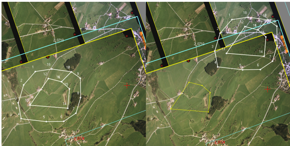
Fig. 209. The resulting ring-shaped polygon and the internal polygon as a separate vector object
