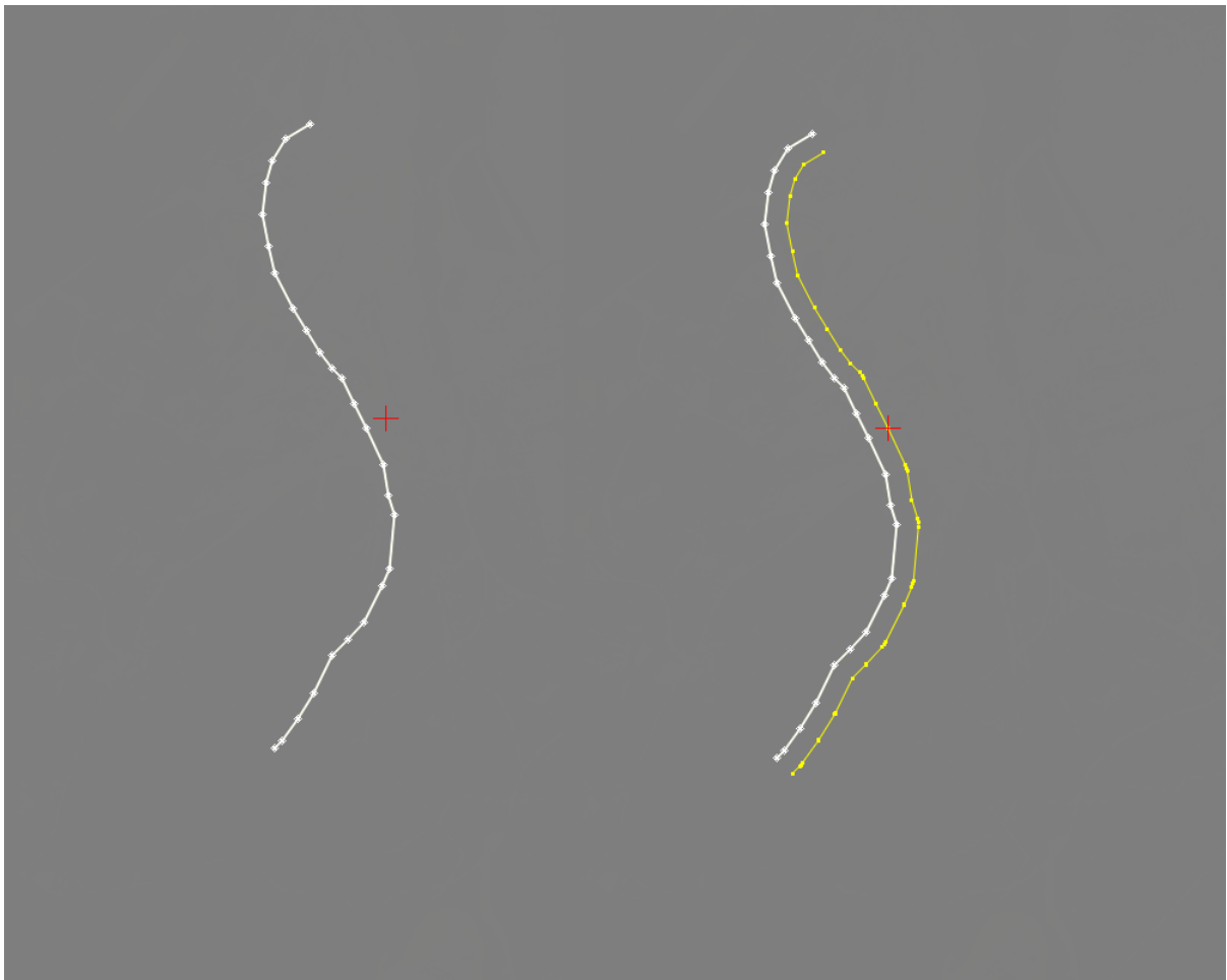
Fig. 179. Steps for creation of the symmetric polylines
