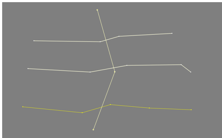
Fig. 205. The “cutting” line and the objects to be cut are selected
